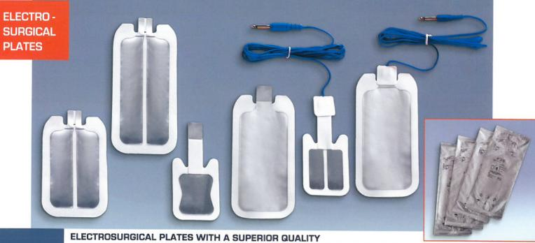
• Made of FOAM suitable to obtain perfect results with all instruments • manufactured and tested in compliance with EN 60601-1/EN 60601-2/AAMI-HF 18 • available with one zone and two zones and REM alarm for adults (adhesive surface 215 sq cm), for children (surface 129 sq cm) and for new born (surface 63 sq cm). All the models are available even equipped with
