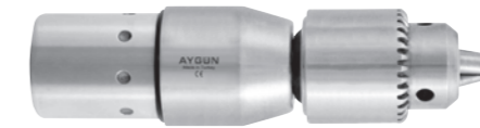
M208-309 Drill attachment with keyed chuck Ø4 mm Cannulated Ø 1.0 mm - 6.35 mm 900 rpm / 4 Nm 30 x 126 mm / 370 g
