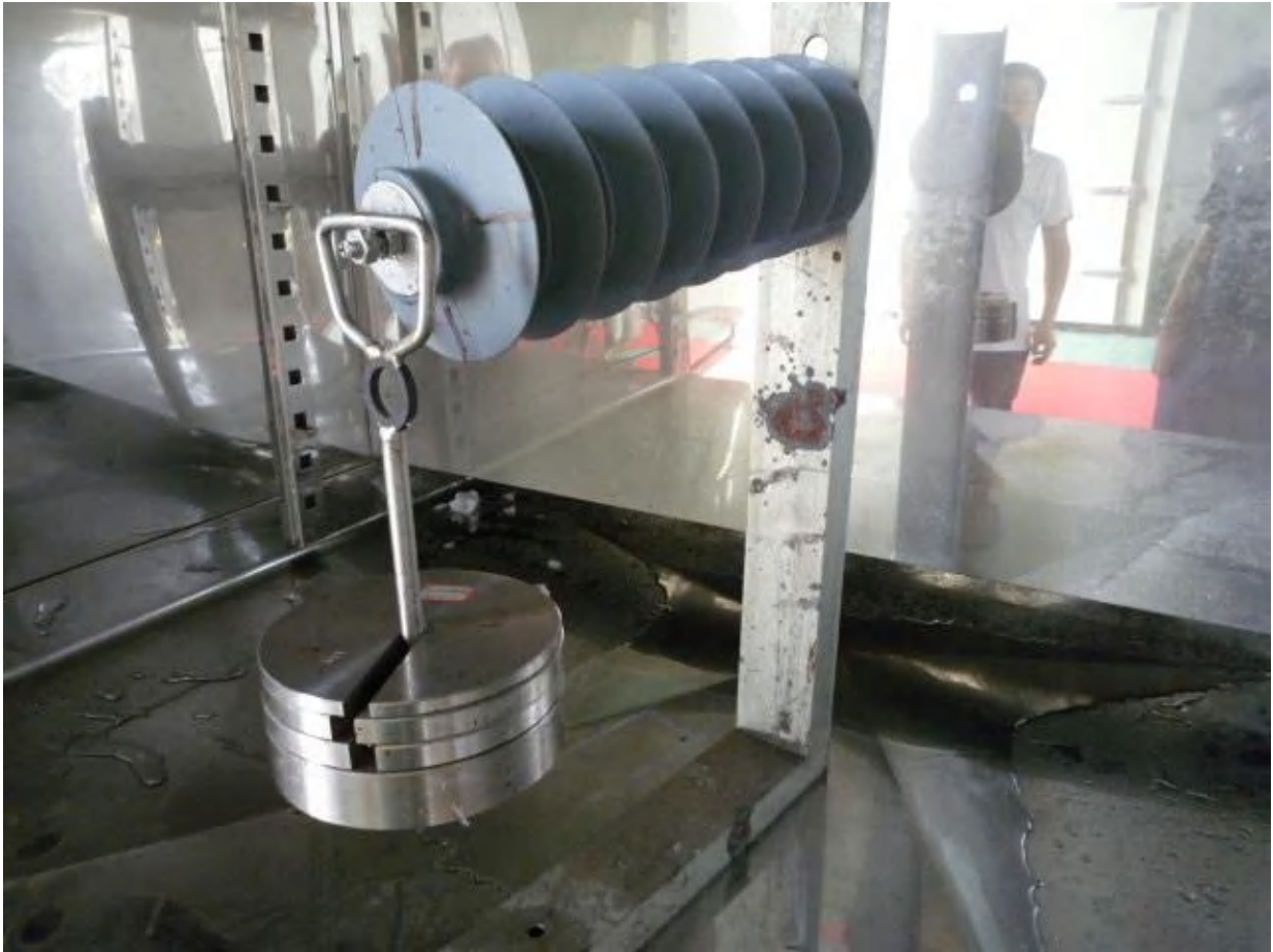
Mechanical and thermal preconditioning test as part of the bending moment test
