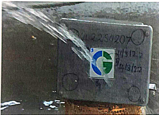
Photograph Number: CPRIBLREATD22T0108P03 During IP X5 – Water Test
