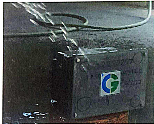
Photograph Number: CPRIBLREATD22T0108P04 During IP X5 – Water Test
