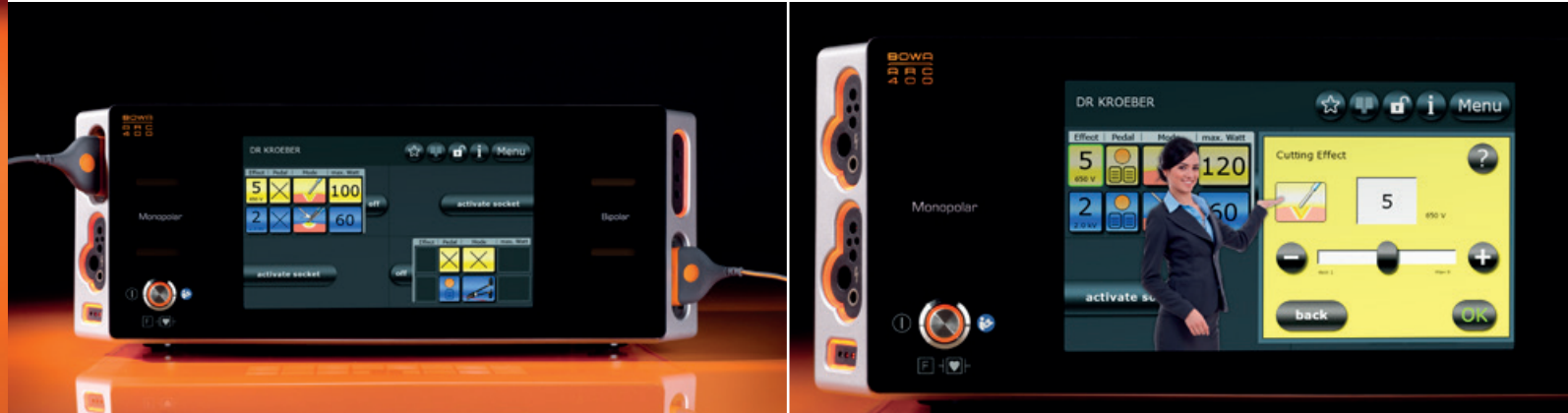
Clarity: Every connected socket – in this photo the upper left and lower right – is clearly assigned to one quadrant of the display
