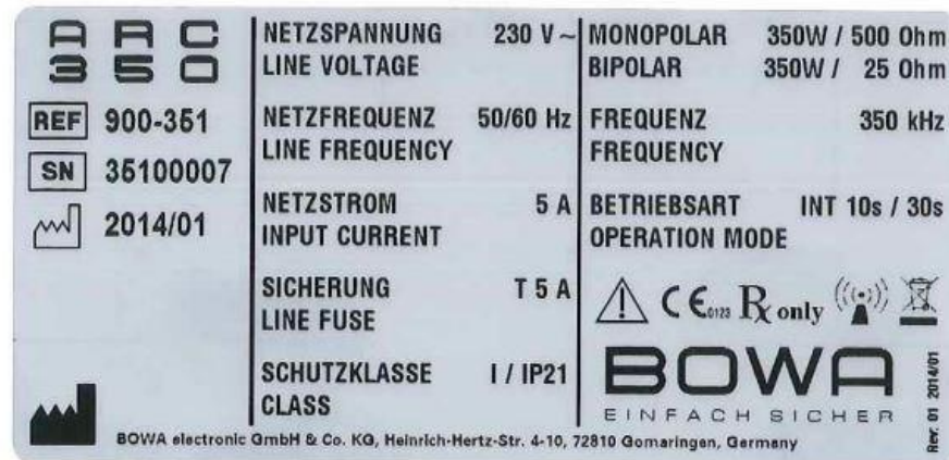
Figure 3-1: ARC 350 rating label
