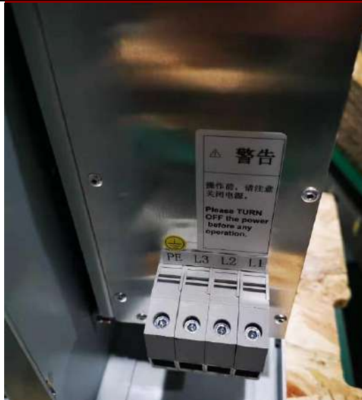
Figure2-3 Three phase-four-wire connection
