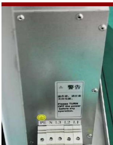
Figure 2-2 Three phase-five-wire connection
