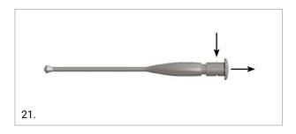
**Step 2:** Position the tip of the cup impactor in the acetabular shell taking care to align the teeth of the impactor with the dedicated sockets near the central hole of the acetabular shell. Screw the central hole of the cup impactor by hand until fully tightened.
