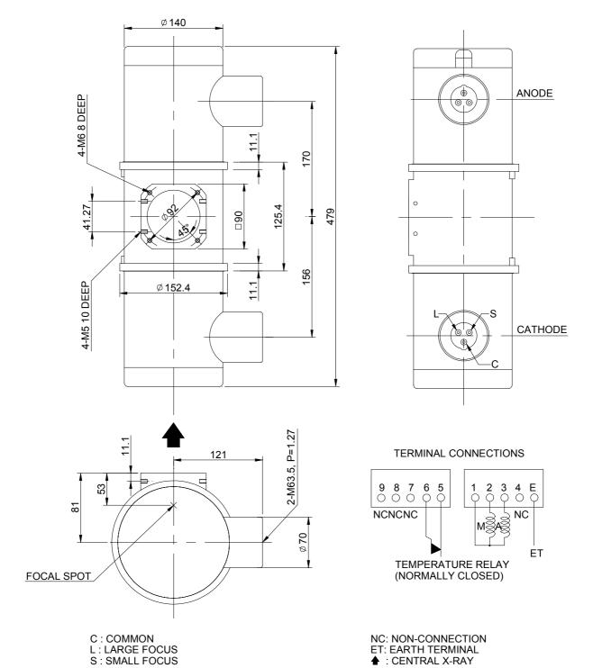
M : MAIN WINDING OF THE STATOR A : AUX. WINDING OF THE STATOR
