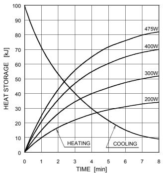
The heating curves are showing examples of average input power to the anode in operation.
