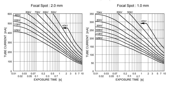
Conditions : Tube Voltage Single-Phase Stator Power Frequency 50Hz
