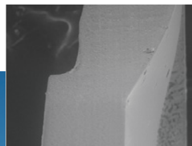
C- Edge profile at Optic-haptic junction. Radius of curvature <10µm.
