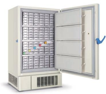
Side-access Freezer Rack · Made of 304 stainless steel for durability and better appearance. · No sharp edges to avoid risk of injury. • Steel plate thickness:combination of 0.5 and 1 mm.  $\cdot$  Side-access design makes it convenient and economic.
