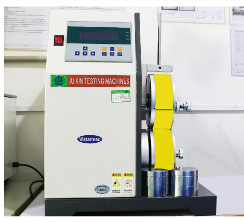
Velcro Lifecycle Testing 魔术贴测试
