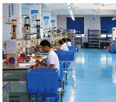
RF Welding Process 焊接作业
