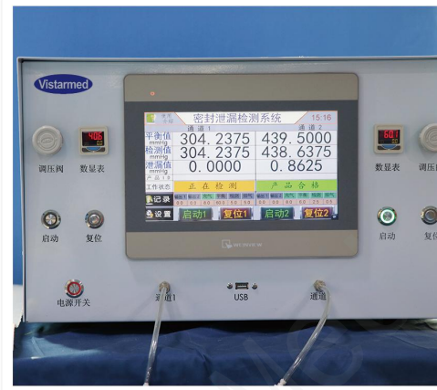
Bladder Leakage Testing 气囊漏气测试
