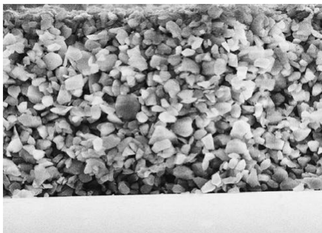
Electron microscope photograph of a cross section through a glass plate with silica layer (magnification x 500)
