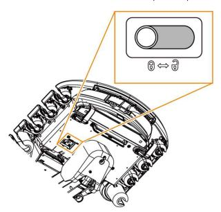
The figure shows the keyboard in a locked state.
