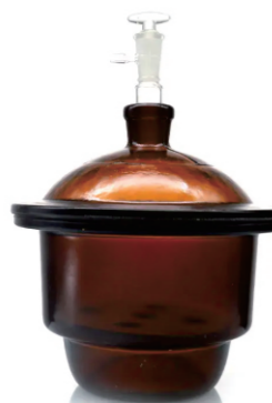
Vacuum desiccator with ground-in stopcock and porcelain plate, Amber glass
