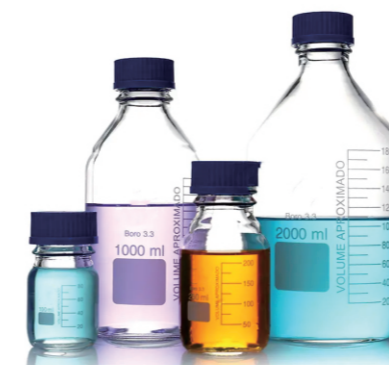
Reagent bottle(Media bottle), with plastic blue screw cap
