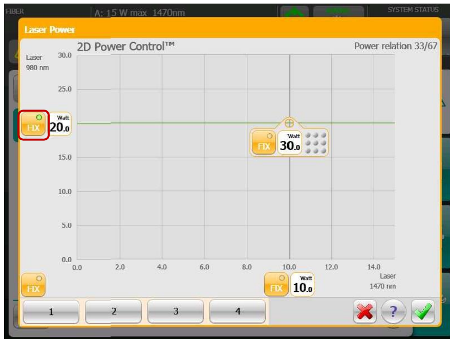
Figure 33: Fixing the power for the wavelength 980 nm on the vertical axis
