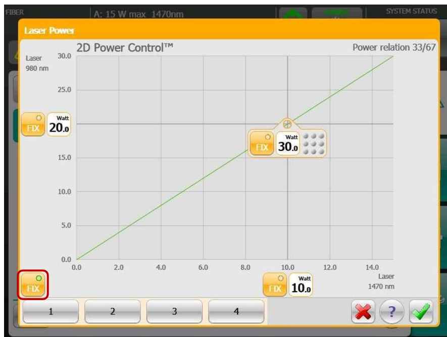
Figure 31: Setting the output with constant relation between two wavelengths
