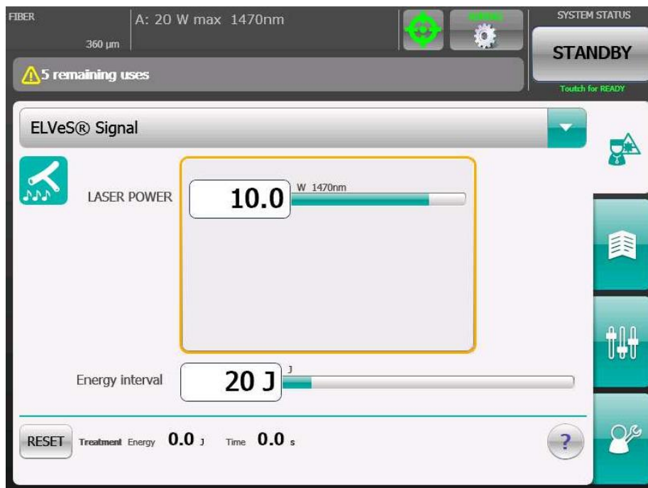
Figure 52: Setting the parameters in ELVeS® signal mode (for devices that emit one wavelength)
