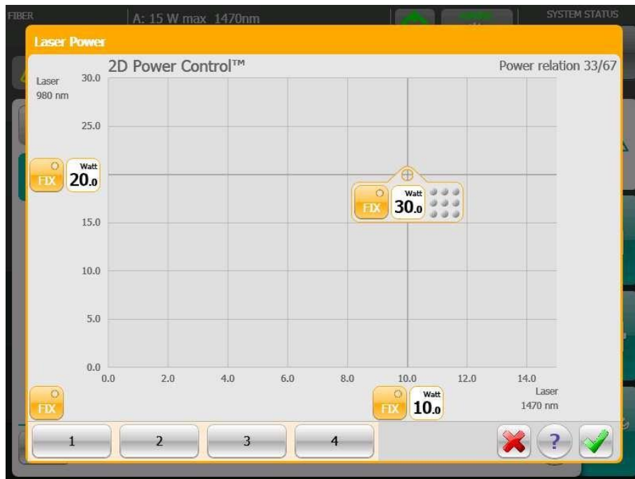
Figure 29: Method 2: Setting the laser power using 2D Power Control™
