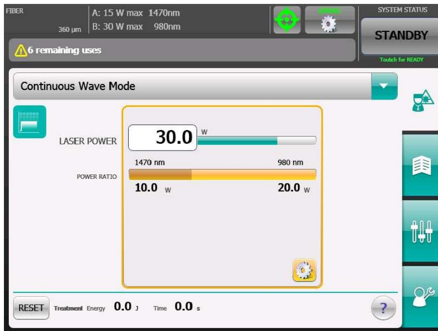
Figure 38: Screen display of Continuous mode CW in standby
