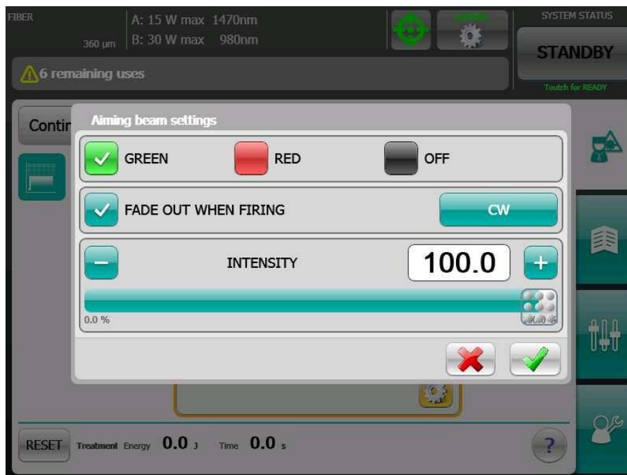
Figure 14: Setting the aiming beam in any application mode by using the PILOT box
