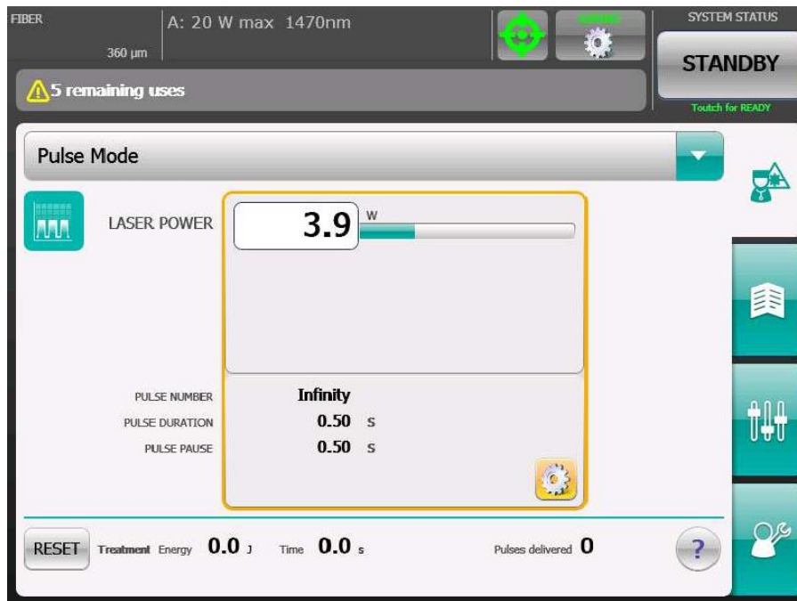
Figure 43: Screen display of Pulse mode (for devices that emit one wavelength)
