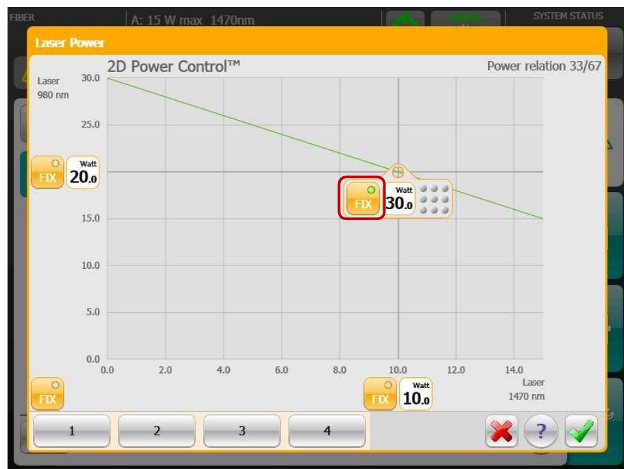
Figure 30: Setting output with constant total laser power output
