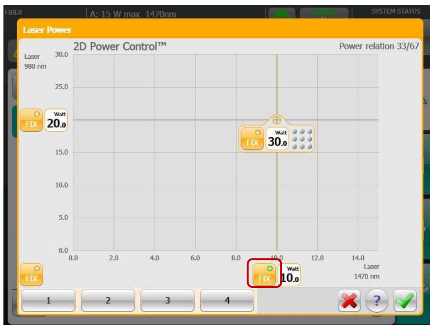
Figure 32: Fixing the power for the wavelength 1470 nm on the horizontal
