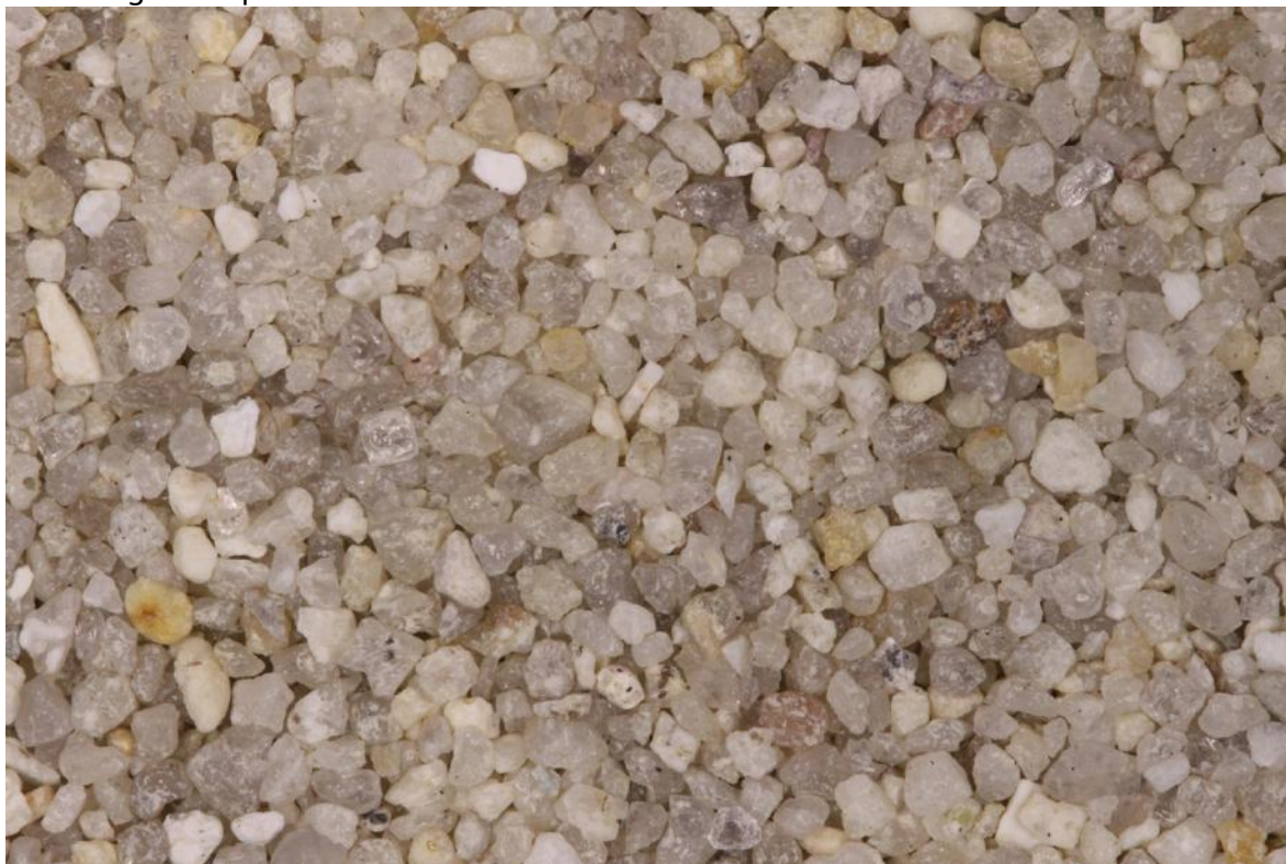
Stabilising Infill - picture
