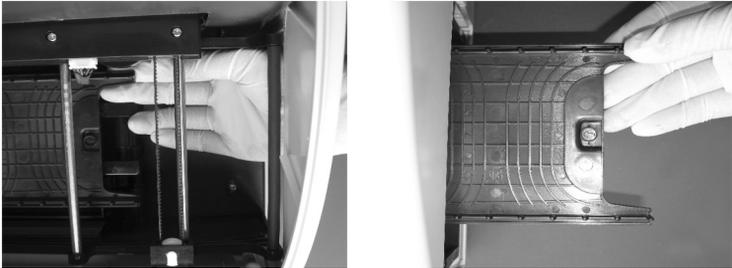
Clean all visible sample deposits with a swab or cotton ball dampened with distilled water. Dry with a clean, dry cotton ball.
