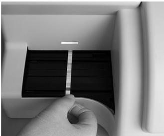
**Note:** Ensure the strip is placed properly onto the Strip Platform. Improper strip placement may cause the Strip Transport to malfunction, resulting in inaccurate readings. Incorrect strip placement may result in a blank test result, displaying only the date, time, and ID number.
