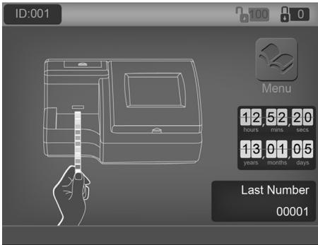
**Note:** If Strip Lockout is provided, the number in the screen upper right corner will display the number of strips remaining for use. If Strip Lockout is not provided, this number will not be displayed.
