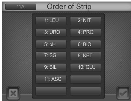
The **Order of Strip** screen is used to select the order in which parameters are displayed on the results screen and on result print-outs. Next to each number, select the parameter desired. "--" means that there will be no parameter displayed for that number. For example, if LEU is selected for position 1, then LEU is the first parameter to appear on the results screen and on the print-out.
