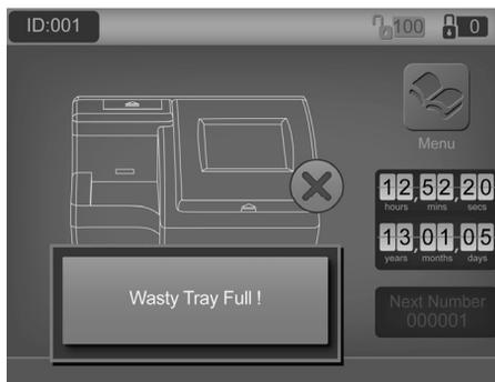
Remove the **Strip Platform and Waste Tray** assembly and empty processed strips as necessary.
