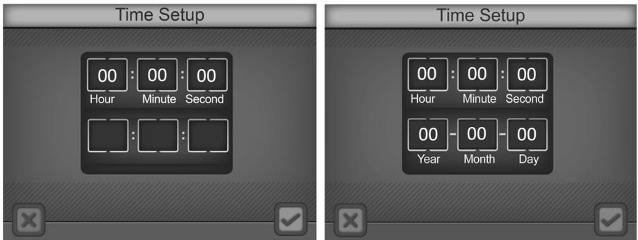
To change any of the **Date** or **Time** settings, press either the name or associated number in the display area. This will bring up the numeric keypad for entering the proper Year, Month, etc.
