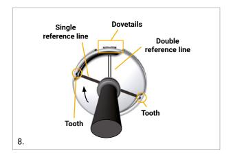
**Step 4:** Correctly couple the two bayonet edges of the impacting ring with the two acetabular shell lips.
