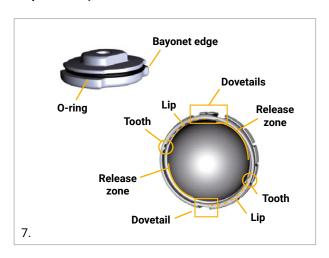
**Step 3:** Position the impacting ring into the shell in the unlocked position (bayonets in the release zones), in order to have:
