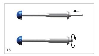
**Step 3:** The assembly is positioned in the acetabular shell by putting two trial liner bayonets in the two release zones and achieving close contact. Lock the assembly into the acetabular shell Versafitcup by turning the impactor handle about 90° clockwise until the two trial liner holes are lined up with the acetabular shell teeth. In the correct position the fixed liner bayonets are completely covered by acetabular shell lips.
