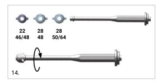
**Step 2:** Assemble the impaction washer with trial fixed liner, introduce and screw the central rod to the last thread in order to stabilize the assembly impactor handle - central rod - trial fixed liner.
