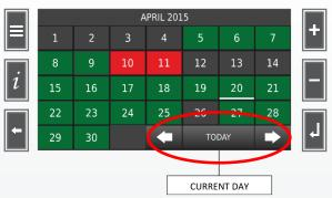
The grey boxes indicate the lack of data, the green boxes the presence of data, the red boxes the presence of a discrepancy. Press the key of the requested day to access the display frame of the daily graph.
