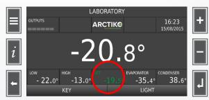
Press the UP to increase the temperature or the DOWN to decrease the temperature. Once the temperature has been set press ENTER to save the new value and exit.
