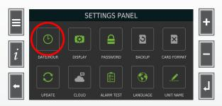
Press SELECT to move the highlight and use UP/ DW to increase/decrease the value selected. The new date/time is saved by pressing the ENTER key with request to confirm.
