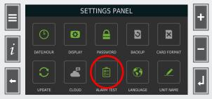
The icon pressure TEST starts the alarm test WITH the following sequences:
