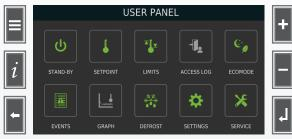
2. If you wish to consult previous logons make a BACK-UP data and open the contents of uSD through the application THERMO CONVERTER where in the last 4 fields to the right are the records accesses with the description by means of the actions carried icons.
