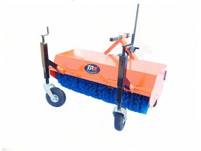
SP 150 sweeper with basket, driven by the PTO shaft of the tractor.
