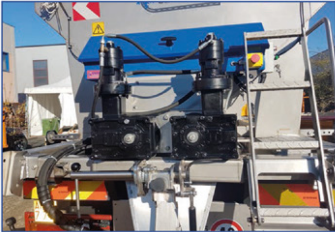
Reducers to decrease the traction force of the augers
