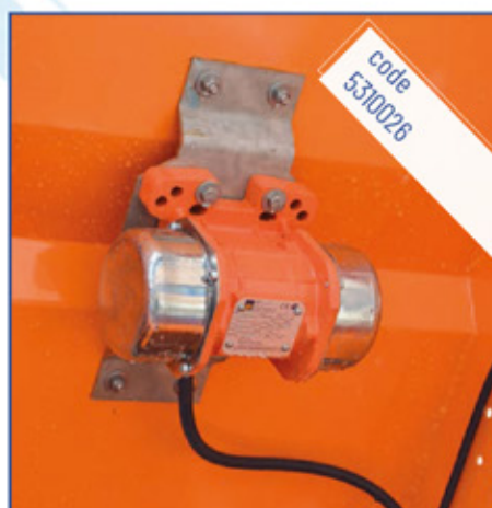
Pair of external vibrators controlled from the push-button panel
