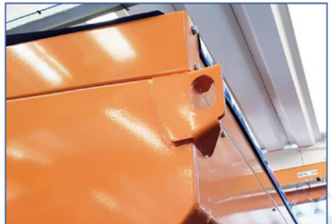
Lifting and fixing hooks/eyebolts (n. 4 in the corners of the hopper)
