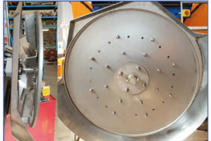
Spreading disc Ø 600 mm with n.º 8 interchangeable and adjustable pallets
