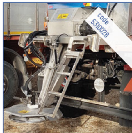
Steel ladder for the hopper inspection
