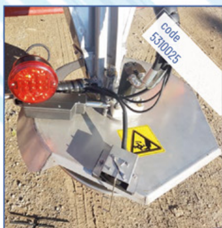
Electric setting of the spreading asymmetry, controlled from the push-button panel
