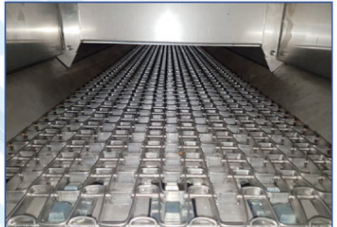
Spreading system through STAINLESS STEEL HONEYCOMB CHAIN
