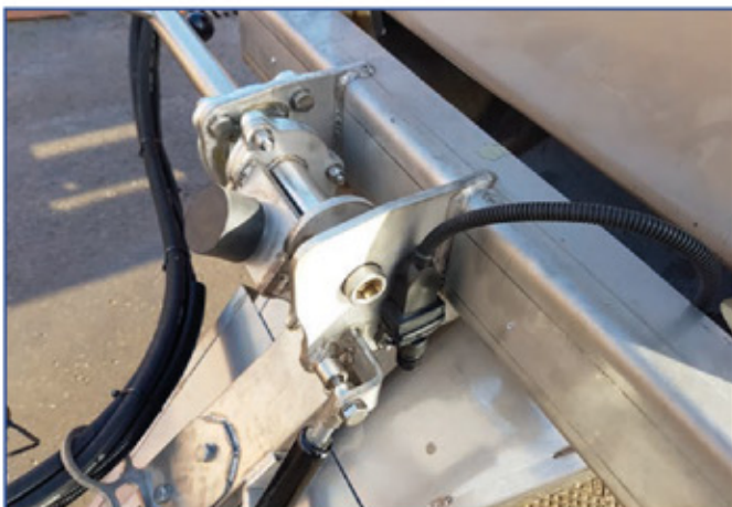
Safety microswitch on the spreading tower
