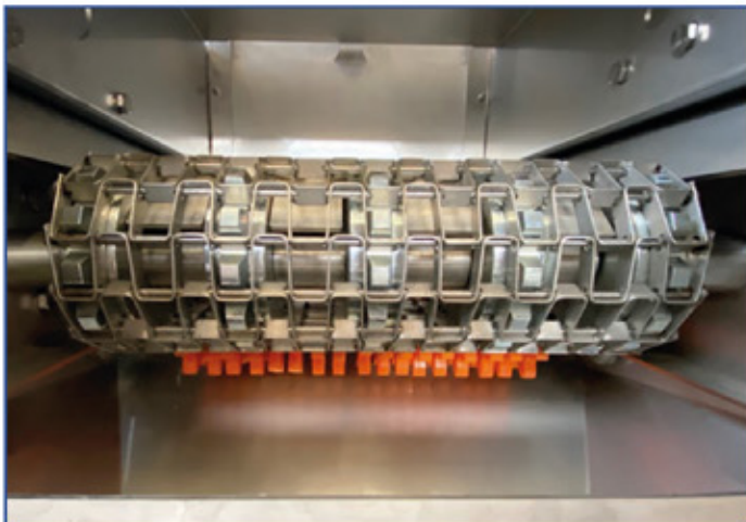
The chain is guided by 5 toothed wheels
