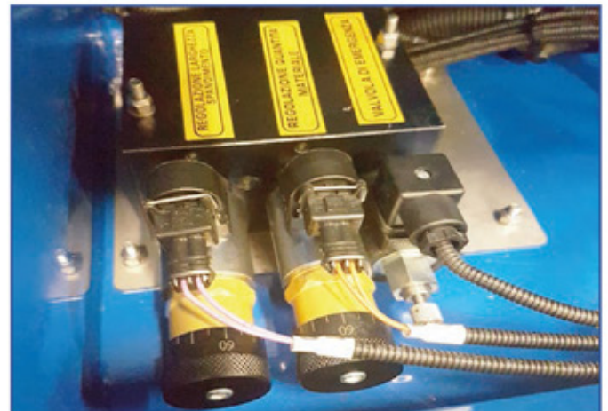
Proportional hydraulic block with the possibility to set the MANUAL operation mode ( emergency )
