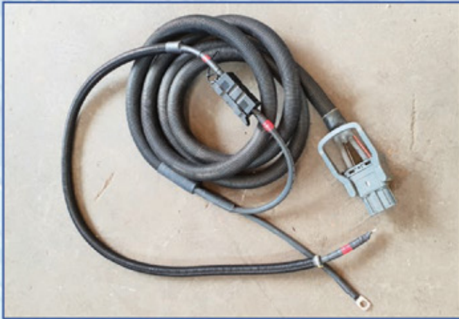
Wiring with plug and fuse for connection to the vehicle battery
