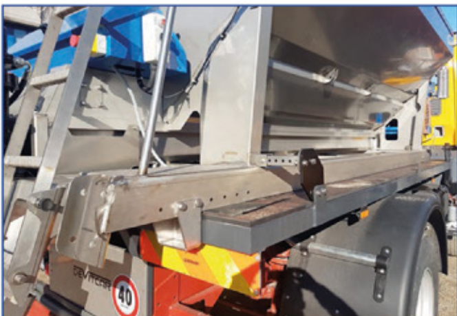
Rear adjustable mechanical stops
