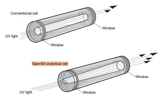
The standard analytical, inert, and LC/MS cells have a path length of 10 mm. The semi-prep and microbore cell path length is 3 mm. The autopurification cell path length is 1.0 mm. A variable path length flow cell (path length 0.15 to 3 mm) is also available.
