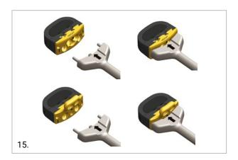
**NOTE:** The Straight Inserter must be attached firmly to the plate to avoid damage to the implant holder or the plate threads. Ensure the correct device positioning by aligning the arrow on the Straight Inserter with the dot laser marked in the front side of the plate.
