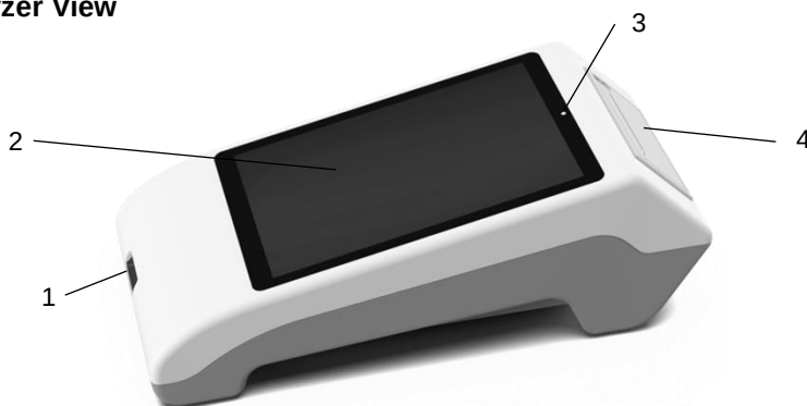
1- Test cassette slot; 2- Touch screen; 3- Indicator; 4- Built-in thermal printer
