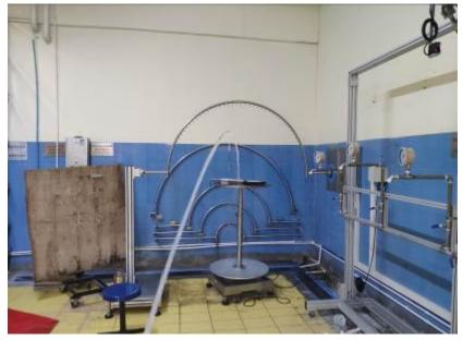
Photo 4 -- During the test of IPX5
