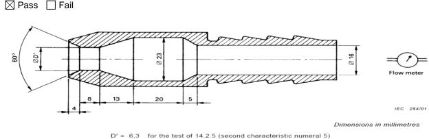
D' = 6,3 for the test of 14.2.5 (second characteristic numeral 5) D' = 12,5 for the test of 14.2.6 (second characteristic numeral 6)
