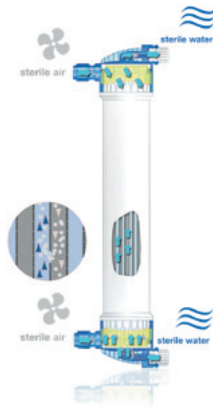
Integrity test: air pressure is applied to the fibre bundle from one side while the other side contains sterile water. If any leakages were present in the membrane, air would pass through the membrane and create bubbles.
