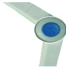
Figure 3.4 – Self-locking button for changing the segments position
