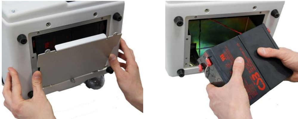
Figure 6.5 – Replacement of accumulator
