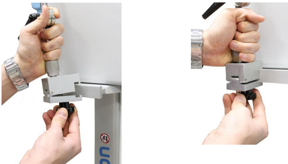
Figure 3.3 – Installation of the supporting arm (circuit holder)
