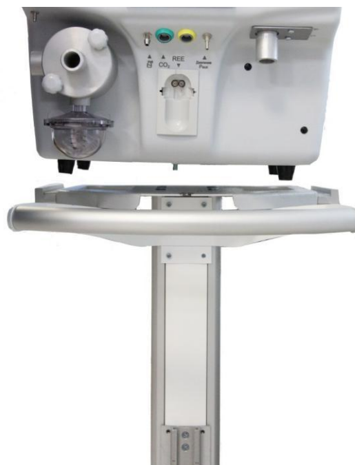
Figure 3.1 – Installation of the electronic unit on the table of the cart
