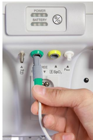
Figure 5.3 – Connecting the CO 2 sensor to the CO 2 connector of the ventilator
