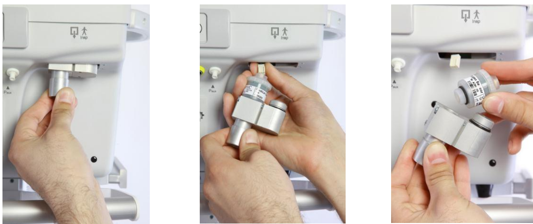
Figure 6.4 – FiO 2 sensor replacement
