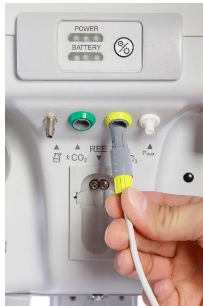
Figure 5.7 - Connecting the pulse oximetry sensor to the ventilator
