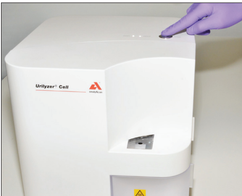
Fig. 26: The Start button on the top of the analyzer is the only interface element you need: press it once and the system feeds a cuvette into pipetting position.
