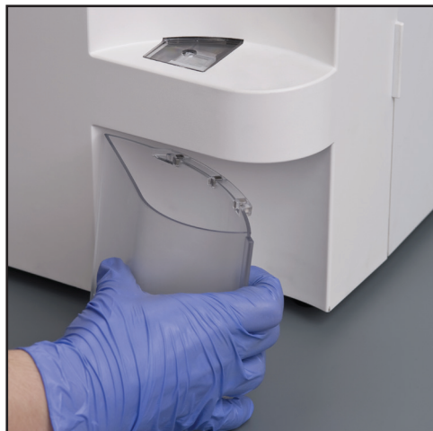
Fig. 30: Do not leave any used cuvettes in the waste drawer at the end of the day. Use the overhanging flap of the waste drawer to grip it and take it off the analyzer.
