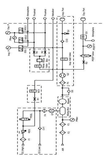
Figure A-1.Pneumatic diagram
