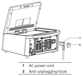
Figure 3-8.Connecting to primary power source
