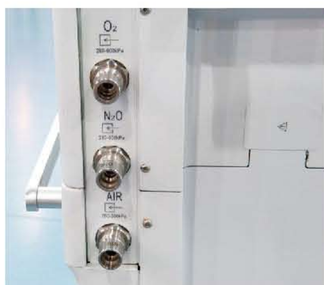
O 2 , N 2 O , AIR PIPELINE SUPPLY INLET
