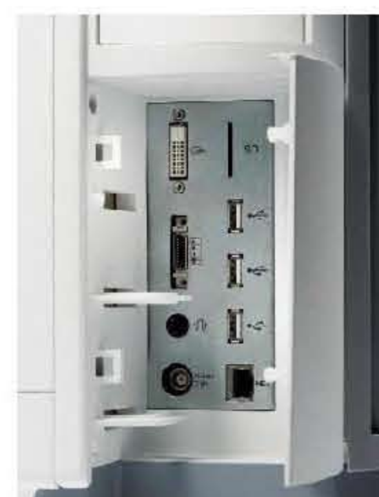
SD socket, multiple USB interfaces, various ports for external devices
