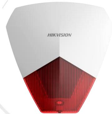
The wired sounder is used to connect to wired control panel, by using 12v output voltage from panel, the sounder can alarm up to 105dB sound. The sounder can be used both internal or external, the LED flash and the sounder indication can be configured separately.
