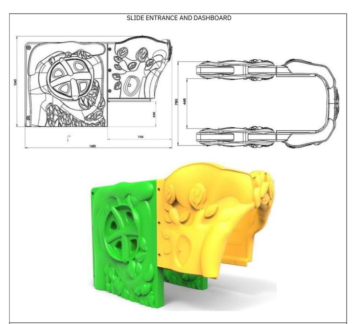
Subject Technical drawing-these are barriers made of metal pipe or polyethylene in order to ensure safe entry to the spiral slide used in the game group, provided that they adhere to the measurements and safety rules.
