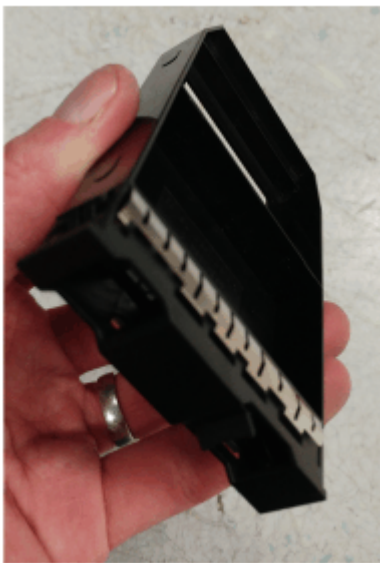
Figure 110. Correct drive blank orientation
