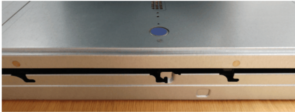
Figure 77. Replacing the node canister cover
