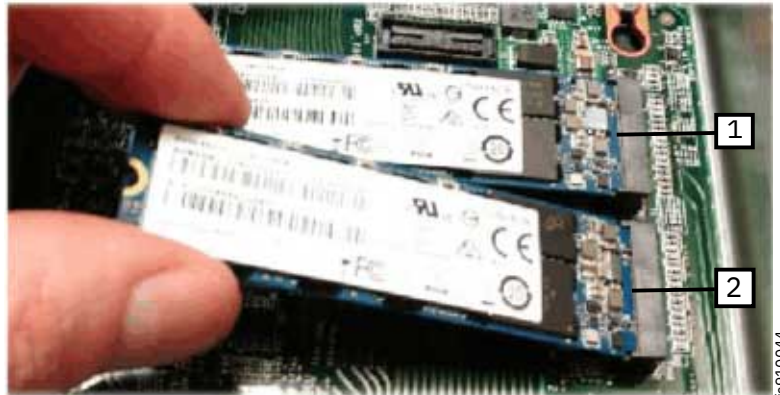
Figure 101. Replacing the boot drive
