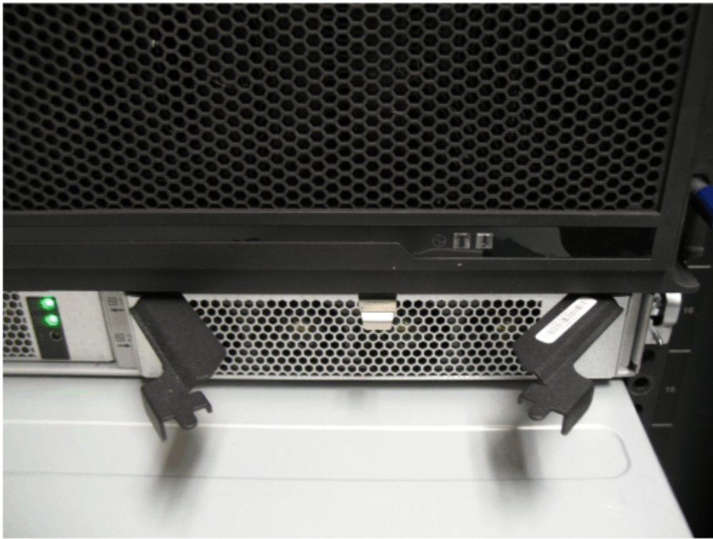
Figure 151. Releasing the power supply handles
