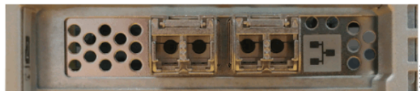
Figure 180. Dual-port 25 Gbps Ethernet host interface adapter ports and LEDs (iWARP)
