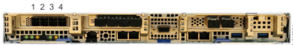
Figure 58. Fibre Channel adapter in node canister 2, adapter slot 1
