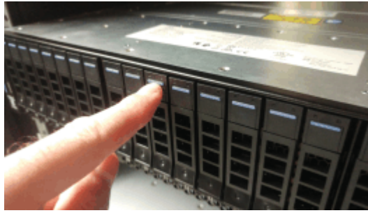
Figure 68. Unlocking the drive and release latch
