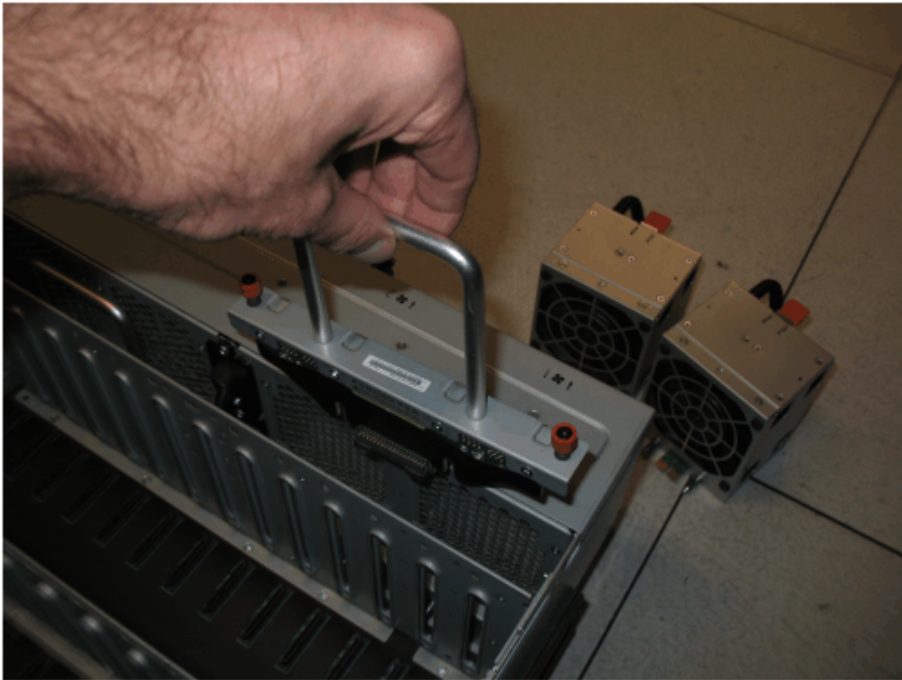
Figure 171. Remove the FIB from the chassis
