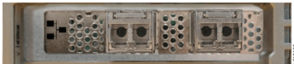
Figure 179. Dual-port 25 Gbps Ethernet host interface adapter ports and LEDs (RoCE)
