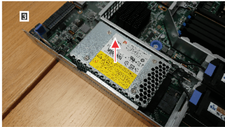
Figure 80. Removing the node battery
