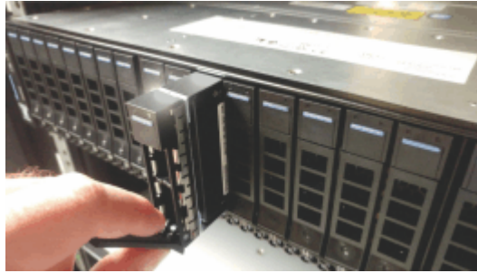
Figure 68. Unlocking the drive and release latch
