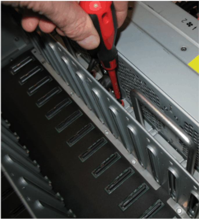
Figure 170. Loosen the FIB screws
