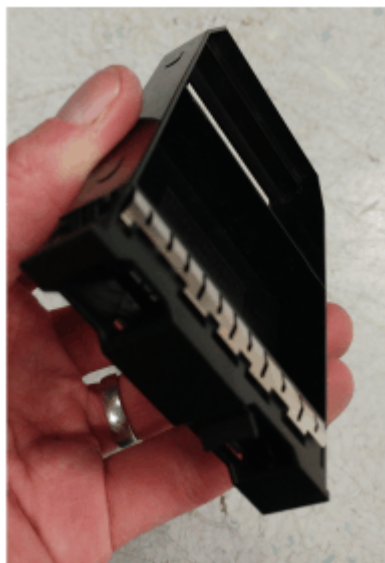
Figure 72. Correct drive blank orientation
