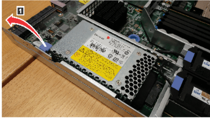
Figure 78. Lifting the latch of the node battery
