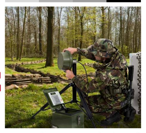
MMD System is a portable protection system using microwave barriers that create invisible detection zones for temporary surveillance of sites considered at risk. Each intrusion attempt into the protected area is detected by the barriers, which immediately sends a radio signal to the MMD control panel located in a guard room or wherever the designated control centre is located. ATTENTION!: Tripods provided only in black color.
