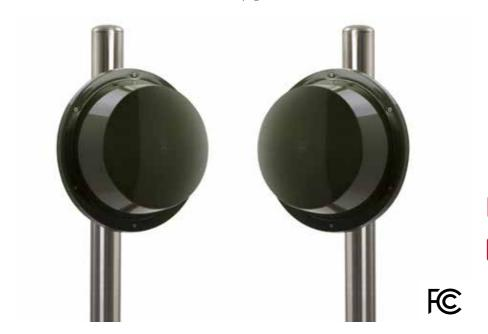
New Digital microwave barrier with parabolic antenna, based on "Fuzzy Logic" analysis of intrusion signal, for range up to 500m, X and K band. The new more powerful microprocessor positively increases its performances both in detection and in false alarm discrimination (POD 99% - FAR 1/unit/year).
