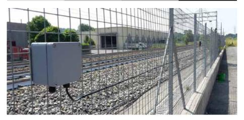
Blackfeet cable is a magneto phonic linear sensor cable specifically designed to provide high performance intruder detection capability when deployed on fences or other barriers like wall used to define the perimeter of a secure site.
