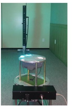
SMF/Lab-CHS photometric is the designed measurement system and manufactured by ARGOS INGEGNERIA to operate in the workshop of AGL airport maintenance department.
