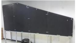
On customer request, SMF/LAB may be delivered with a dedicated portable dark room, composed by wooden panels, which includes the control console.
