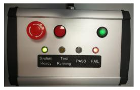
Steps of measurement process may be also controlled through a dedicated console, particularly when the system is operated in the dedicated darkening tunnel.
