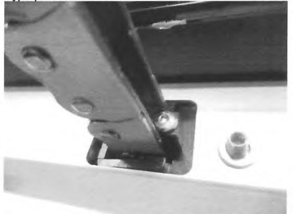
Picture 10 Chain outlet on drive housing after 20,000 cycles
