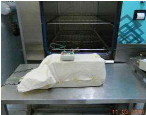
Here the relative humidity is measured by a blade sensor (exemplary picture)
