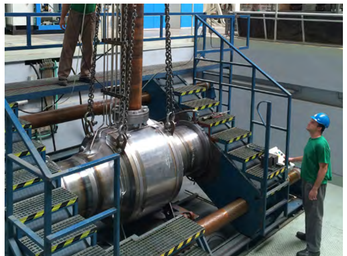
Pressure test of ball valves at our workshop
