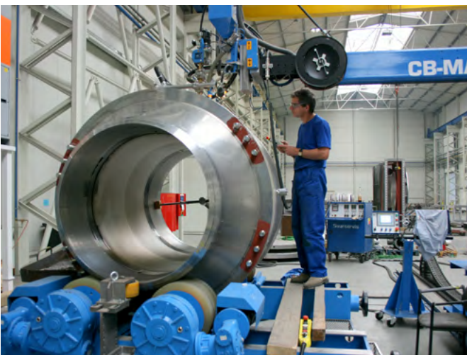
Automatic welding of ball valves DN 1400
