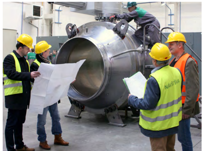
Inspection of ball valves DN 1400 for Eustream, Slovakia
