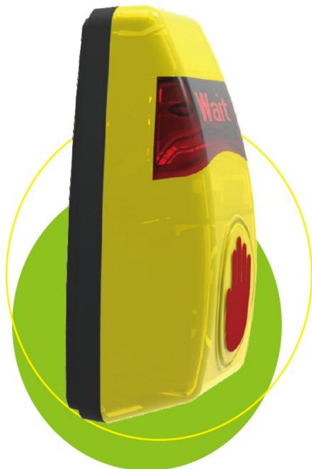
The housing is made of **polycarbonate**, which is self-extinguishing, impact resistant and retains its mechanical properties over a wide temperature range. Polycarbonate is also highly resistant to chemicals such as gasoline, lubricants and alkaline hydrocarbons. These features make the button extremely resistant to environmental conditions as well as vandalism.
