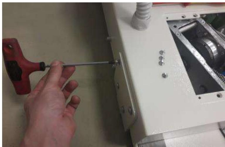
9. **ROTATIONAL CARRIAGE ONLY:** Reinstall the motor assembly. Leave the cover of the access port off.
