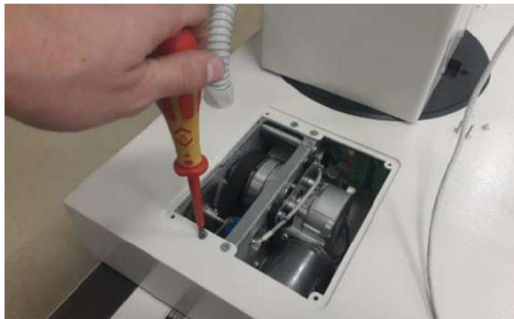
4. **ROTATIONAL CARRIAGE ONLY:** Remove the 4 screws holding the motor drive assembly.
