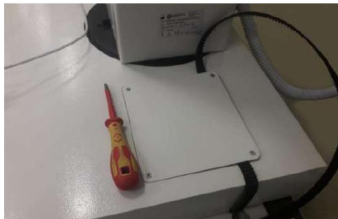
14. Mount the threaded plate here similarly to that of the left side and install the rear roller bracket assembly. At this point, the drive belt is flattened, but is NOT YET TIGHTENED.
