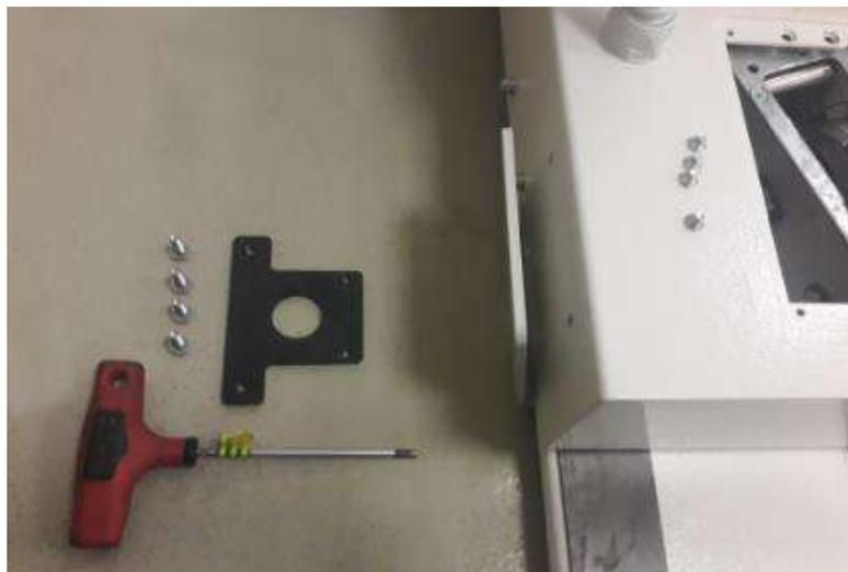
8. On both sides of the floor carriage: insert the T-shaped threaded plates inside the carriage. Mount and **pull up the brackets firmly** until the rollers inside reach the roller track, then tighten the roller brackets mounting screws.
