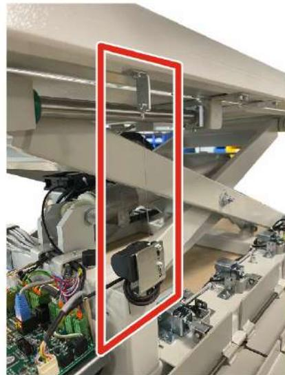
The wire of the sensor is disconnected to prevent damage during shipment.
