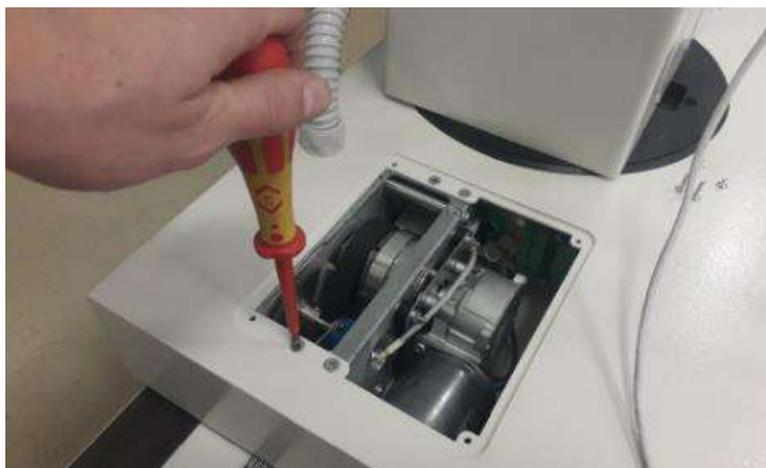
10. CAREFULLY move the tube stand into a position that corresponds to the factory preset position of the longitudinal potentiometer. The position is slightly asymmetrical. Use the values as indicated in Figure 26.
