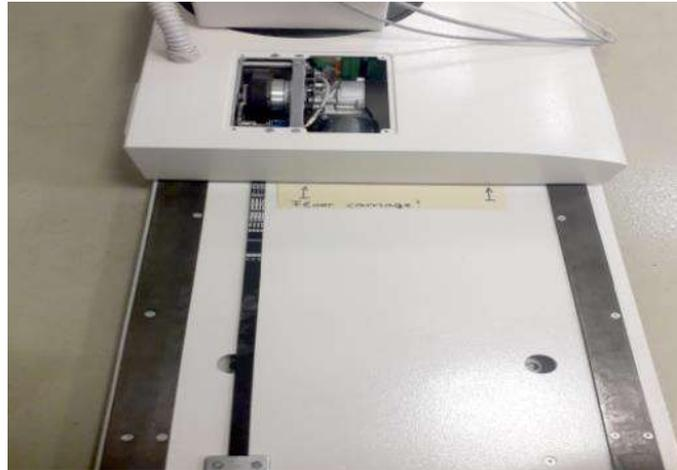
13. Remove the right side service access cover. Repeat the drive belt flattening and securing on the right hand side.
