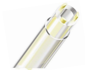
Bilayer construction of Perifix® ONE showing three x-ray contrast stripes embedded in the polyamide inner core
