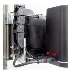
Fig. 19: Cable connections of PolFlash XE and camera to ATBM Tower (viewed from the left and right)
