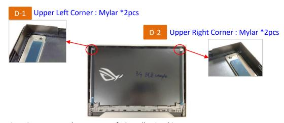
Step 3: Remove release paper of LCD Adhesive \*2pcs.
