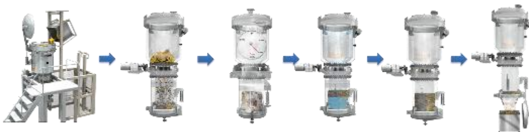
1.Loading 2.Shredding 3.Sterilization 4.Cooling 5.Vacuum 6.Unloading
