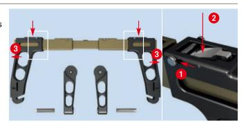
The outer rails can be separated from the inner rail by pressing the buttons on the outer rails and pulling the two rails apart (3).
