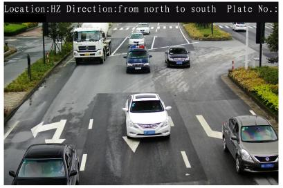
Figure 8-3 Overlay Above the Picture
