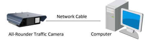
Figure 1-1 Connecting Directly
