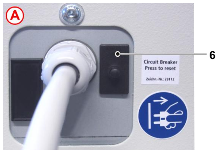
Fig. 4: Detailed view A - Mains power input bracket
