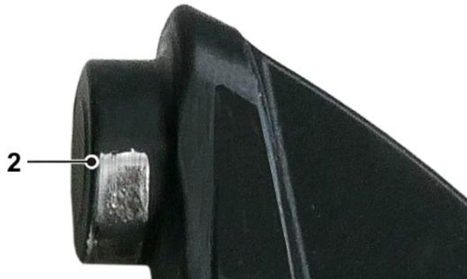
Fig. 10: Load-bearing bolt with completely worn-off anti-friction coating – greasing required
