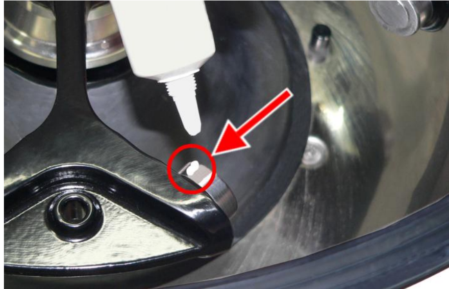
Fig. 38: Sufficient quantity of grease for one bolt
