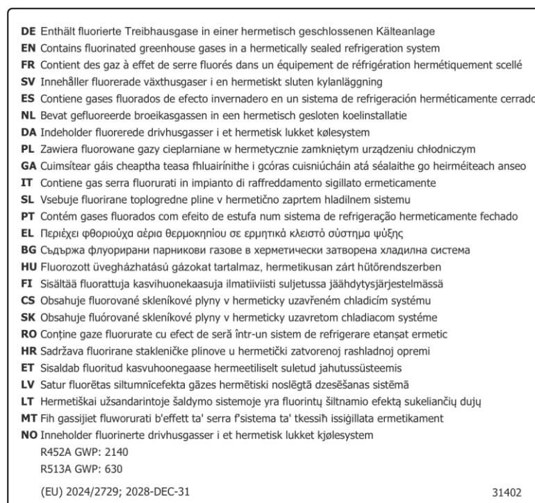
Fig. 6: F-gases label in compliance with the implementation regulation (EU) 2024/2729
