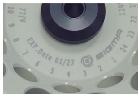
Fig. 7: Different service life – engraving on the bucket/rotor
