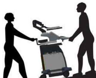
Moving the system on incline
