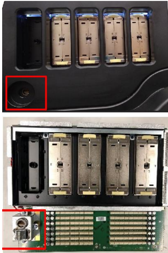
Figure 5-8 Pencil Probe Connector
