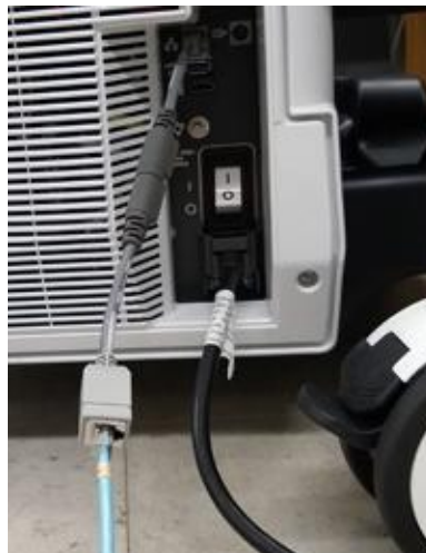
Figure 3-31 LAN cable with protection cable (example)
