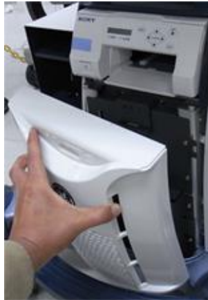
Figure 10-3 Remove the front cover
