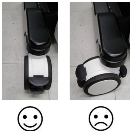
Figure 4-10 Caster position for Swivel lock
