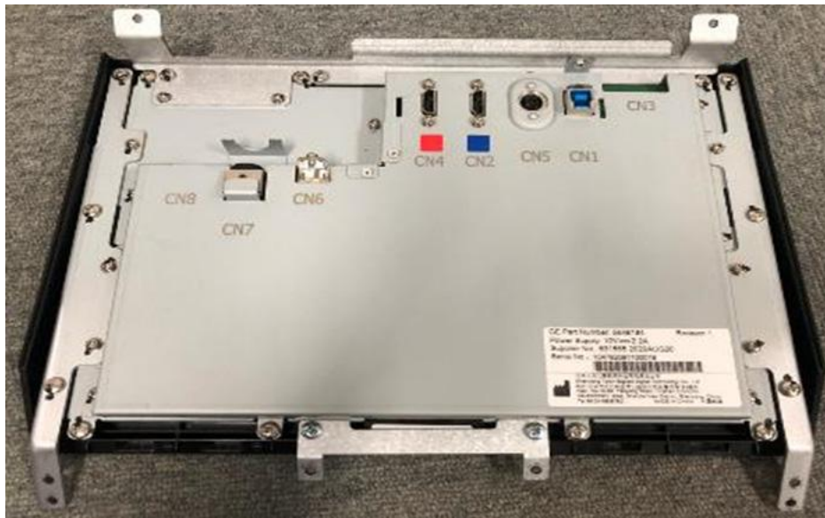
Figure 5-22 Upper Op Panel/Touch Panel Assembly Connections
