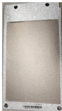
Power Supply Bracket cover with absorber sheet
