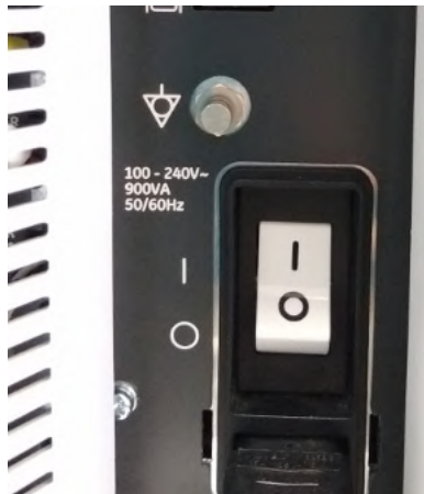
Figure 10-2 LOGIQ Fortis Main Power Supply Grounding Point
