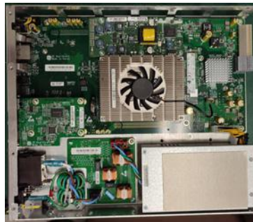
BEPS2 Assy with absorber sheet (The image in BEPS2 assy)
