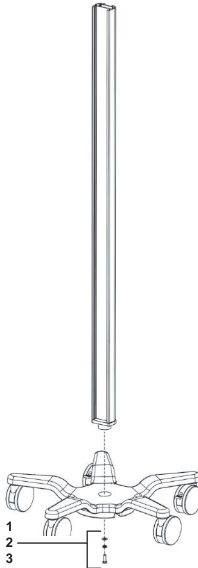
Figure 8-7 Post into Base - (1) 5/16 fLAT Washer, (2) 5/16 Lock Washer, (3) 5/16-18 x 1 inch Screw - Roll Stand only
