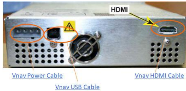
Figure 5-30 V Nav Option HDMI Routing
