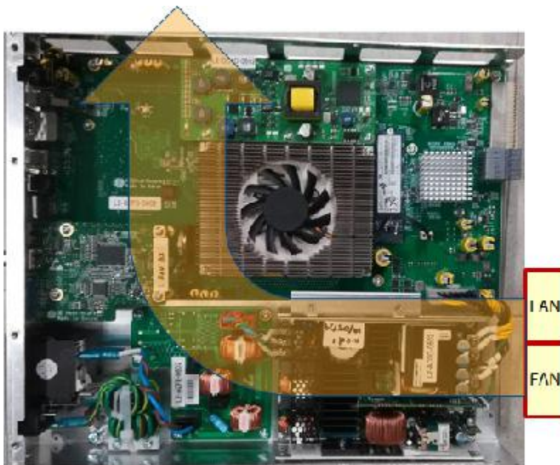
Figure 5-25 Cooling Air Flow of Power Supply
